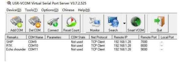
Note 1: The serial port number can be customized according to the actual situation, as long as it does not conflict with the computer's existing serial port. Note 2: The port is associated with the serial number of each set of ship control and cannot be modified. For the specific port number, please refer to the instructions in the accompanying documentation.
